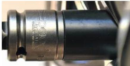
**paoli** impact sockets for alloy wheels application allow not to damage the wheel as they have a black teflon part (detached from the metal socket) that can rotate. This feature enables the tyre repainer to work with no worries and avoid marking or scratching the wheel, also in the presence of grains of dust that in the rotation of the socket could damage the wheel.
