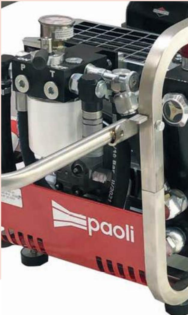
DYNO-M GASOLINE power pack with 6 Hp gasoline engine – recoil starter is designed to guarantee the minimum weight and easy transportability. The machine is available in two configurations of hydraulic power: 20 L/min @ 95 Bar or 12 L/min @ 160 Bar.
