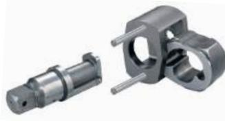
The jumbo system produces a single impact for each cycle. This system is mainly used for 1/2 inch small impact wrenches. This hammer mechanism is extremely strong and performing.
