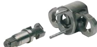
The twin-hammer system produces a double impact for each cycle on both sides of the shaft. The use of 2 opposite hammers allows to obtain a balanced impact. It is mainly used for 1/2 inch impact wrenches.
