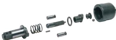
The pin-clutch system produces a single impact for each cycle. The strokes are made by two pins which are pitched directly on the shaft. This creates a balanced impulse and a lower vibration level compared to the other systems.
