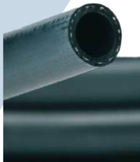
Polyurethane hoses extremely flexible and light; spark proof, ideal for light devices; black coloured; working pressure: 10 bar - 145 psi. Suggested for 3/8" e 1/2" impact wrenches.
